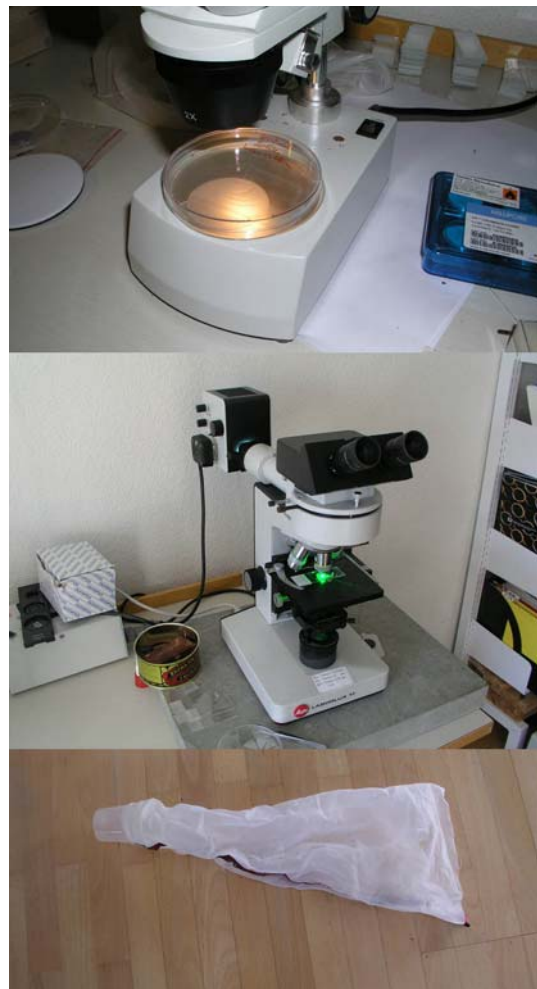
Figure 1. Microscopes and plankton net (80 \mu m) used in the survey
