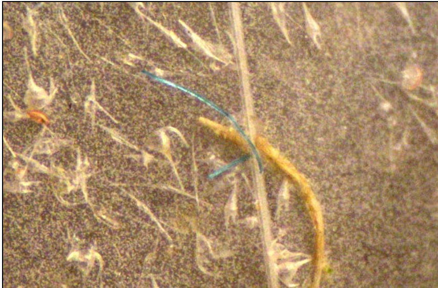
Blue plastic fibre, diameter ~20 \mu m
